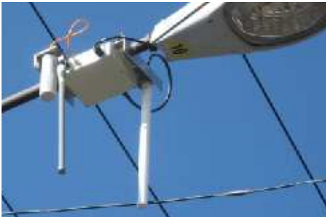
Figure 4. Argos sensor node deployed on a street lamp. The thick antenna pointed down on the right is for the 900MHz backhaul radio, and the thinner antenna on the left for the 802.11 sniffer. The node is powered from the streetlight.
