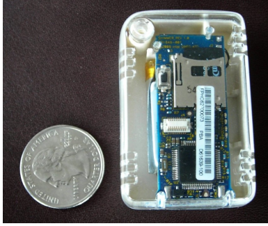
Figure 1: The SHIMMER wearable sensor platform.
