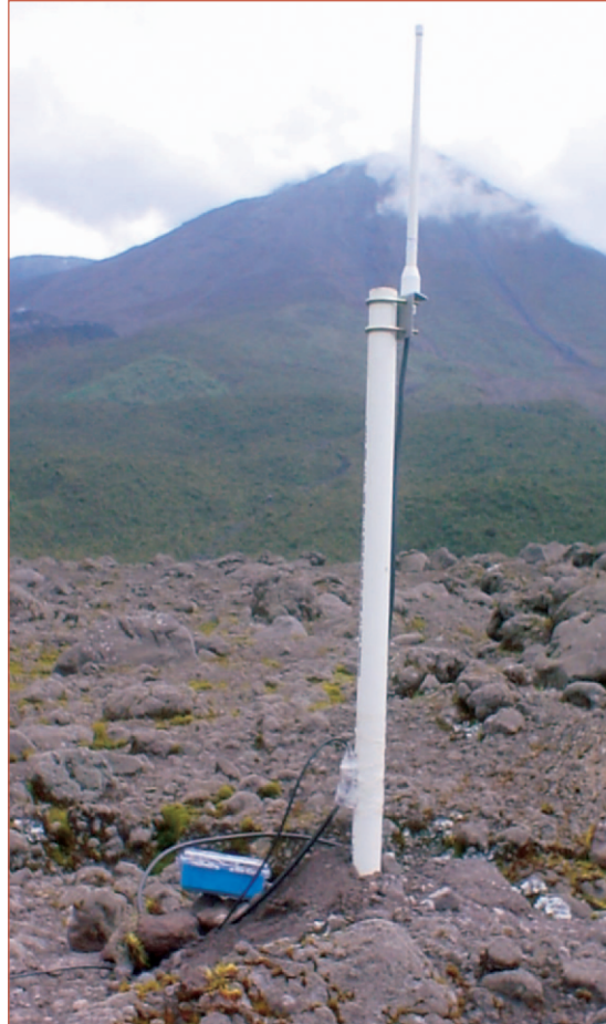
Figure 2. A two-component station. The blue Pelican case contains the wireless sensor node and hardware interface board. The external antenna is mounted on the PVC pole to reduce ground effects. A microphone is taped to the PVC pole, and a single seismometer is buried nearby.
